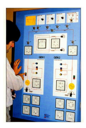
This combination of conventional instrumentation and real-time graphic displays PC managed enables a wide range of exercises to be conducted, including the study of real/reactive power, paralleled generator load sharing, excitation control and power factor.
