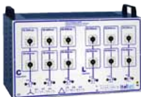
Mod.4020-20LC Load for 3-phase alternator Load inductives & capacitatives; Variable with 20 steps : 5% ÷100%; Power: 50VA÷1000VA Triphase / monophase; (monophasé with 60 steps);
