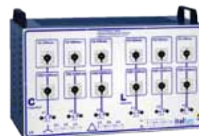
Mod.4020-110LC Charge for triphase alternator · Inductive & capacitive load variable with 3x 1%÷110%; · 3Ph: variable with 110 steps from 1% to 110% · Power: 10÷1000VA; Triphase / monophase; (monophasé with 330 steps);
