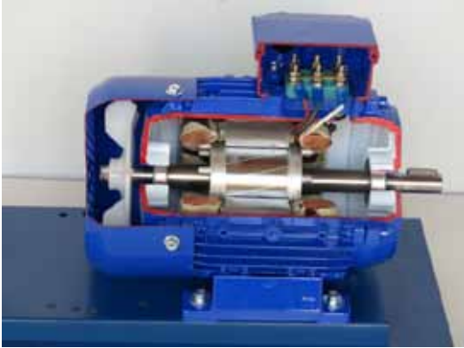
MOD.3040 Three Phase Squirrel Cage Motor
