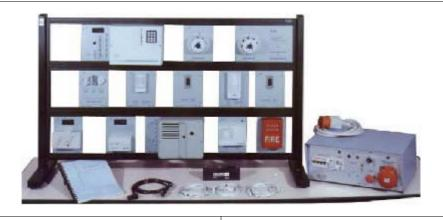
The "ALARM KIT "IT.0377.IT consists of an harmonious and functional modular unit appositely carried out for the study of the electrical alarm plants employed in the Civil and Industrial fields.
