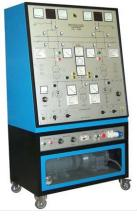
The A generator can also be used as a motor in order to simulate pumping operation or execute the phasing of the other branch. Between the first and the second generator there is a beating signal lamp on the translation bars.
