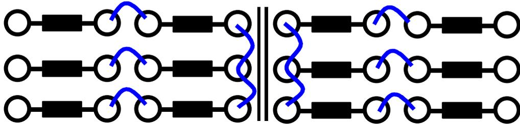
**Transformateur triphasé - Connections triangle-triangle**
