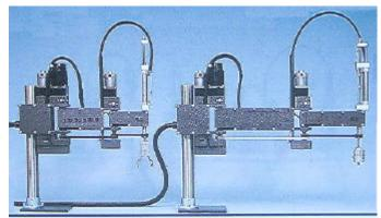
The Serpents may be programmed from the computer either by setting the data for each axis or by steering the arm by hand using the lead-by the-nose buttons. Alternatively the Serpent EC will follow the hand-held control pendant or simulator.
