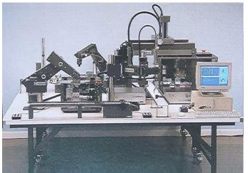
The belt is now incremented to take the part to the pick-up point of Mentor 1 ready for lifting and then placing in the motorised vice of the mill. The vice and parts centraliser now position and clamp the part ready for the mill to run a machining cycle selected upon the dimensions of the part.
