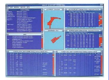
An advanced feature of WALLI for Windows is DDE (Dynamic Data Exchange) which enables it to share data with other Windows programs that support DDE. This enables other manufactures equipment such as vision systems to be operated in conjunction with the work-cell.
