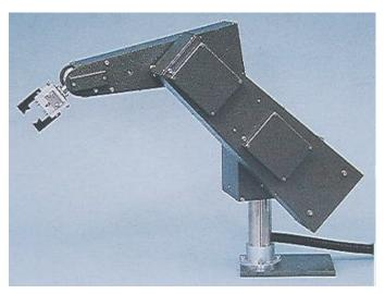
Each axis is powered by a stepper motor with encoder feedback to provide closed-loop control. In the controller there is one microprocessor to monitor the positions of the axes, two more to control the motors and another one to supervise the first three and to communicate with the host computer.
