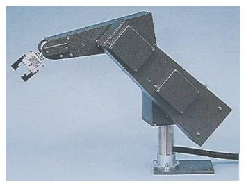
Each axis is powered by a stepper motor with encoder feedback to provide closed-loop control. In the controller there is one microprocessor to monitor the positions of the axes, two more to control the motors and another one to supervise the first three and to communicate with the host computer.
