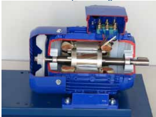
Mod.3040 Three Phase Squirrel Cage Motor
